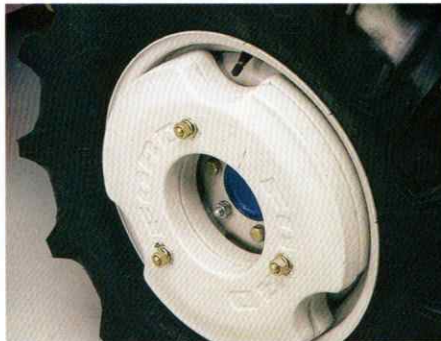
Rear wheel weights help maximize traction and stability.
