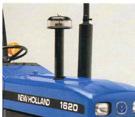
A precleaner can be installed for improved performance in dusty conditions.
