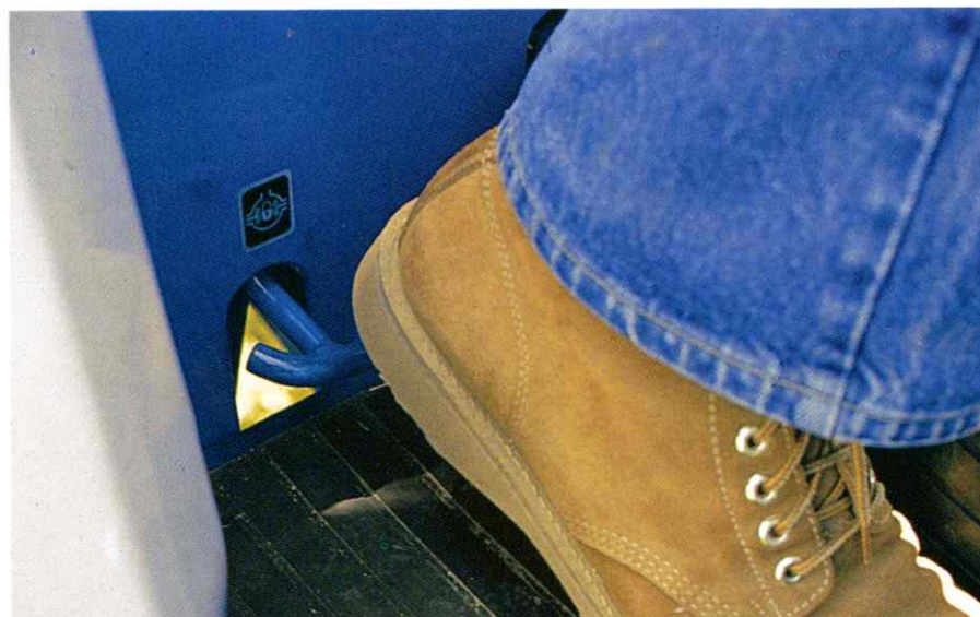
Differential lock offers more positive traction in slippery conditions with a touch of the heel pedal.
