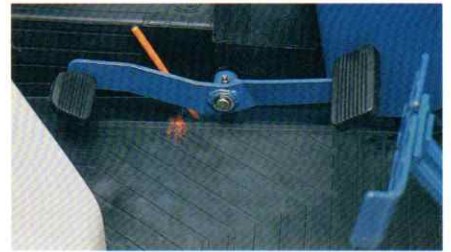
The hydrostatic transmission lets you change direction and speed by depressing the toe-heel pedal.
