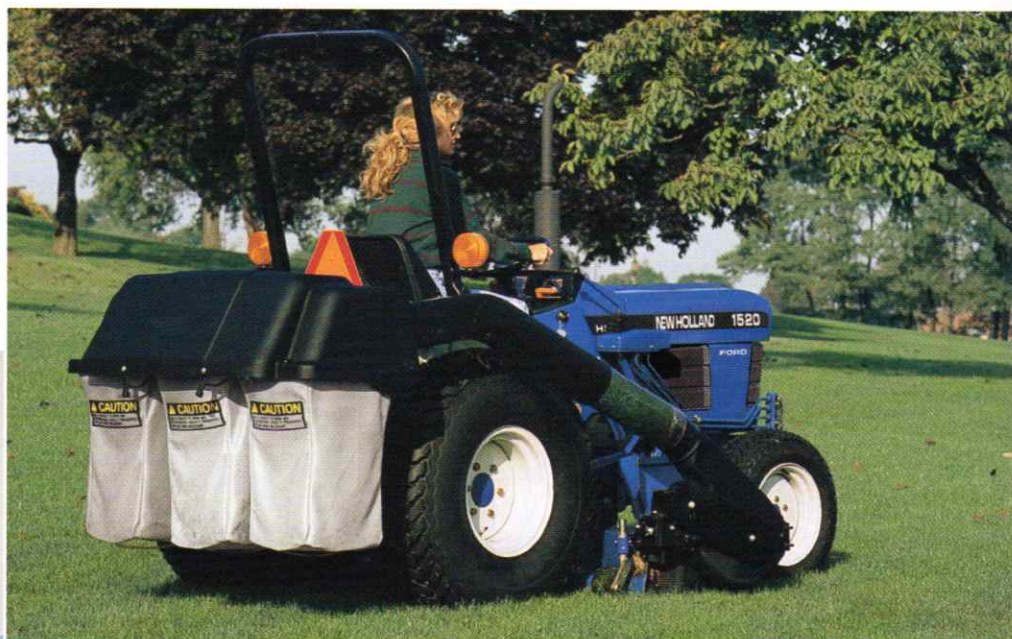
The handy three-bag collector system has an ample 10 cu. ft. capacity (9.75 bushels).
