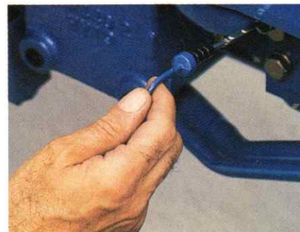
Check the oil level without raising the hood.
