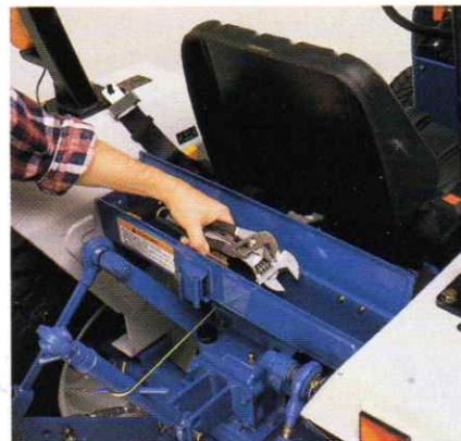
A handy toolbox provides a convenient storage location for the PTO cap and tools used for implement attachment. (Standard on all models except the "1215" and "1715").
